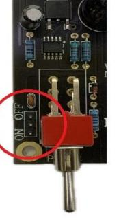
The jumper here can set the bottom 4 LEDs to be ON or OFF.
