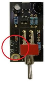
The jumper here can set the bottom 4 LEDs to be ON or OFF.
